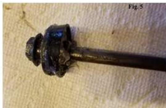
**Figure 5.** Orientation of seal and washer are reversed after modifications.
