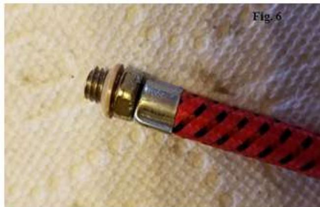
**Figure 6.** Location of built in check valve prior to modification.
