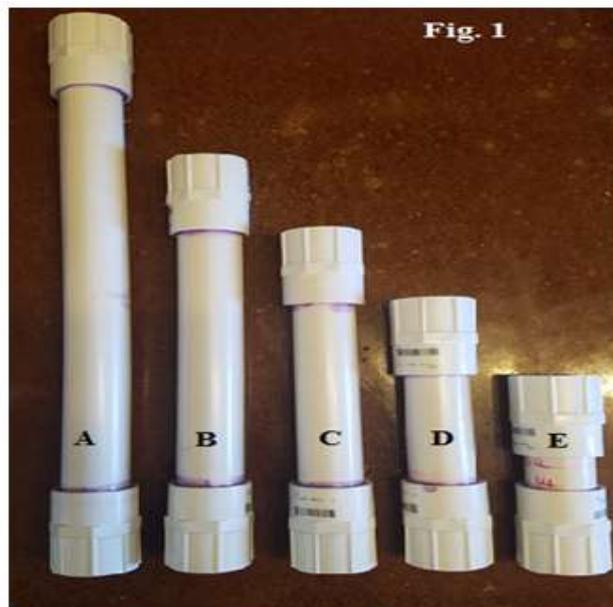
**Figure 1.** Fixed chamber volumes: 12.54 in<sup>3</sup> (A), 8.52 in<sup>3</sup> (B), 6.46 in<sup>3</sup> (C), 4.56 in<sup>3</sup> (D), and 2.69 in<sup>3</sup> (E).
