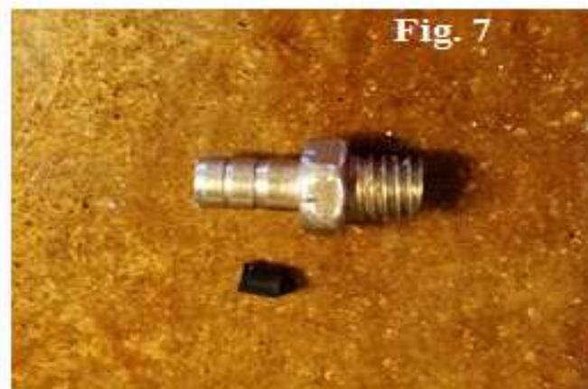
**Figure 7.** Removal of built in check valve
