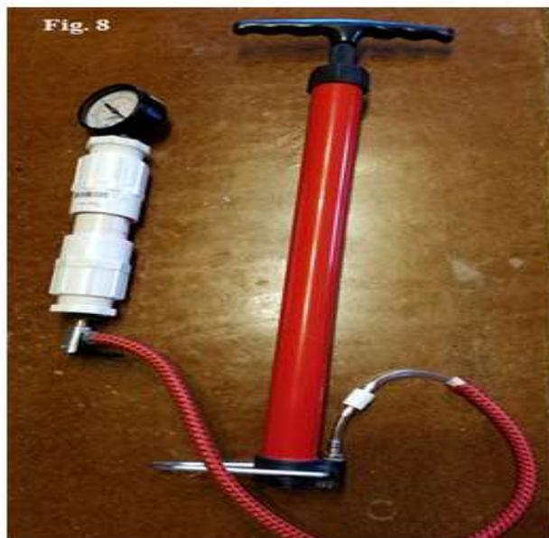
**Figure 8.** Modified bicycle pump with replaced check valve connected to a fixed volume chamber.
