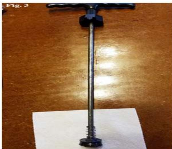
**Figure 3.** Bicycle stem removed exposing washer and seal.
