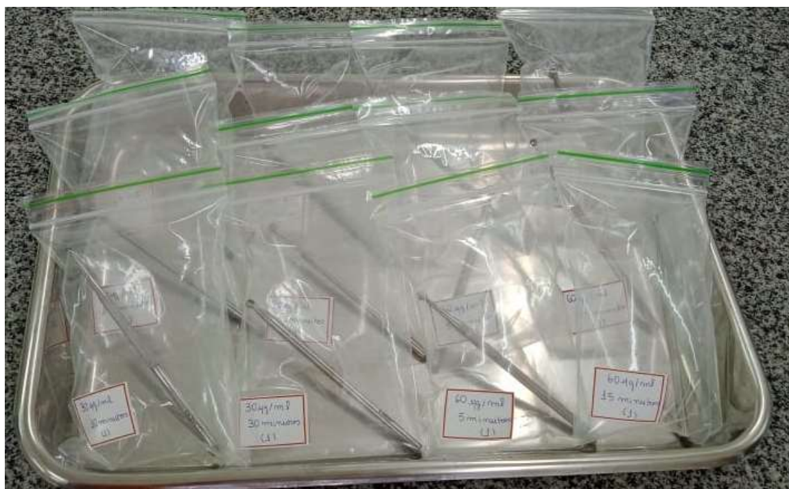
Figure 2: Ozone bags containing curettes exposed to different exposure times and concentrations.
