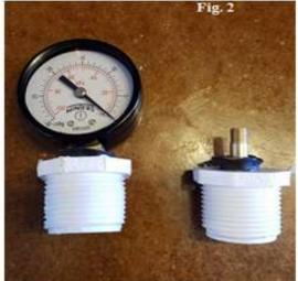
**Figure 2.** Vacuum Gauge and Schrader Valve attacked to PVC threaded caps.
