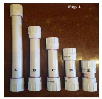
**Figure 1.** Fixed chamber volumes: 12.54 in<sup>3</sup> (A), 8.52 in<sup>3</sup> (B), 6.46 in<sup>3</sup> (C), 4.56 in<sup>3</sup> (D), and 2.69 in<sup>3</sup> (E).
