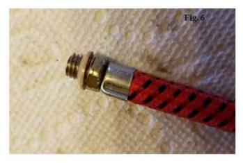
Figure 6. Location of built in check valve prior to modification.
