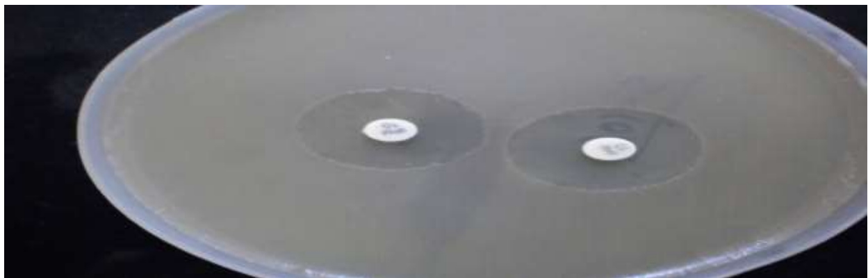
Figure 1: KPC -Combined disc diffusion test: a) Imipenem (b) Imipenem+EDTA. Test negative for KLEBSIELLA PNEUMONIAE CARBAPENEMASES production
