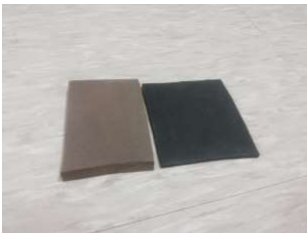
Figure 1 showing the Ethyl vinyl acetate(brown) and microcellular rubber (black) cut in 2 small rectangular pieces of equal size.
