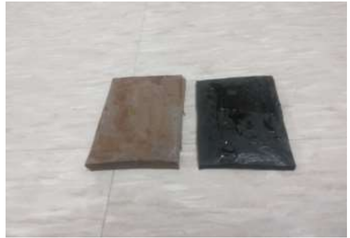
Figure 2 showing application of rubber adhesive to both EVA and Microcellular rubber piece.
